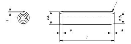
a Swaged chamfer at both ends.
